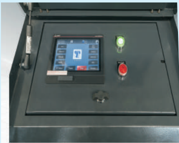
HMI Self diagnostic feature for easy trouble shooting, warning, cautions, alerts, etc. HMI display feature lot size programmed & cut completed, program number in use, current drawn by saw motor, etc.
