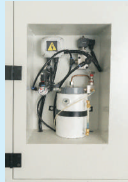
Micro mist oil used as coolant is clean, eco-friendly and highly effective. No water-flood coolant is used thus no spillage and no dirty shop-floors.
