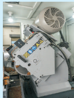
Rigid construction of the Slant type cutting head, moves on state of the art Linear Motion Guide ways which facilitates very accurate and nearly friction less movement. Because of the use of linear motion guides the life of cutter is
